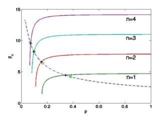
FIG. 5. (Color online) Fitting procedure. The four continuous colored lines represent the solutions of Eq. (2), i.e.,  $\beta_n = \mathcal{F}(p)$ , for the first four vibrational modes. The blue dashed-dot line satisfies Eq. (12), i.e.,  $\beta = \mathcal{V}(p)$ . The solutions for Eq. (5) are the intersection points between these lines (black plus signs). The fitting procedure minimizes the absolute distance between these intersection points with the simulated data (green circles).
