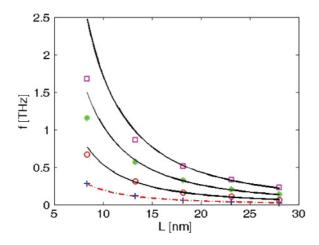
FIG. 2. (Color online) First four vibrational modes as a function of length. The plus signs, circles, asterisks, and squares are for modes 1–4, respectively, and the continuous and dashed-dot lines are derived from Eq. (3).
