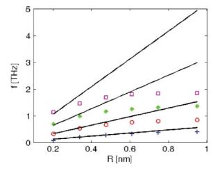
FIG. 3. (Color online) First four vibrational modes as a function of radius. The plus signs, circles, asterisks, and squares are for modes 1–4, respectively, and the continuous lines are derived from Eq. (3).
