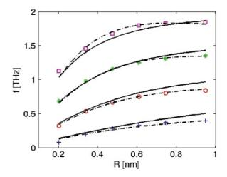
FIG. 7. (Color online) First four vibrational modes as a function of radius. The plus signs, circles, asterisks, and squares are for modes 1–4, respectively, continuous lines are derived from Eq. (5) with  $E=3.5~{\rm kG}=3.83$  TPa and  $h_e=0.67~{\rm \AA}$ , and dashed-dot lines are solutions for the same equation with the same bending and shear rigidities but with  $0.4 \leqslant h_e \leqslant 0.6~{\rm \AA}$ .
